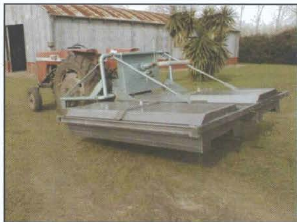
Fig. 20. An injection type boiler in Argentina. Steam is forced into the soil through a platform.
