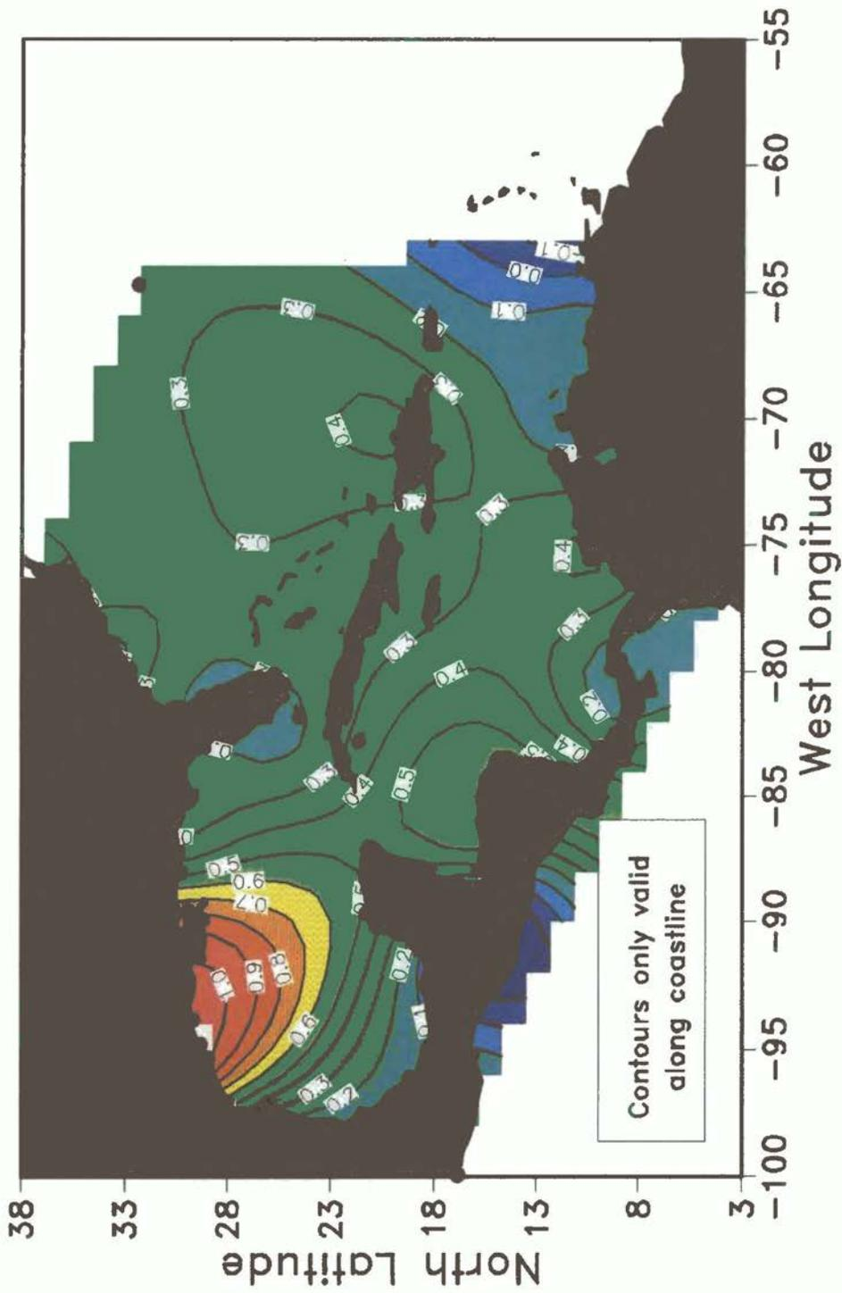
**Fig. 9.8** Distribution of linear trends in annual mean sea level for stations (dots) with more than 10 years of record during the last 60 years. Of the 51 stations used, eight are from the Pacific Ocean and are not included in Table 9.2.
