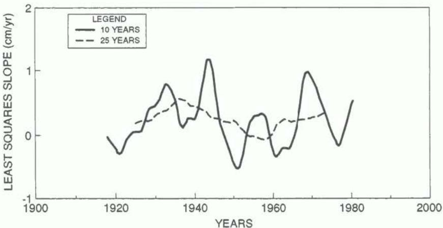
**Fig. 9.9** Linear least-squares slope of Key West sea level (see also Fig. 9.7) calculated as a function of both record length and central year.
