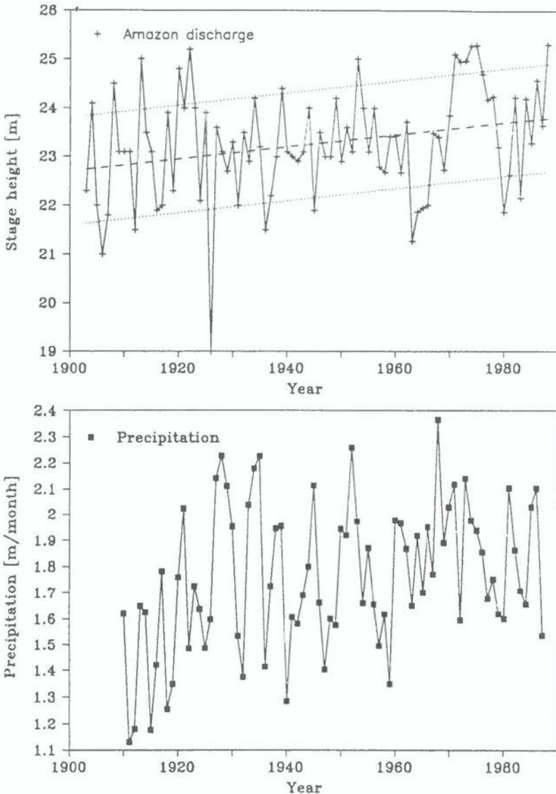
**Fig. 8.3** Time-series of annual mean stage height values (m) (1903–1988) and annual mean precipitation estimates (m/month) (1910–1987) at Manaus on the Amazon. The linear trend ( $\pm$  SE of the slope) shown for the Amazon stage height was obtained by least-squares regression (see Table 8.1).
