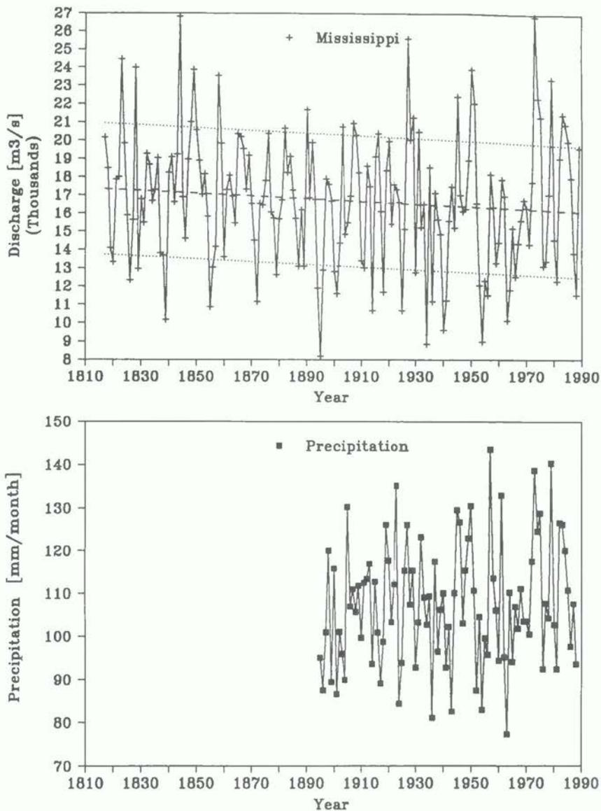
**Fig. 8.9** Mississippi. Time-series of annual mean discharge values ( $\text{m}^3\text{s}^{-1}$ ) at Vicksburg on the Mississippi (1817–1989) and annual mean precipitation estimates ( $\text{mm}/\text{month}$ ) (1895–1988) along the Mississippi valley. The discharge did not show a trend in spite of massive human development along the Mississippi banks.
