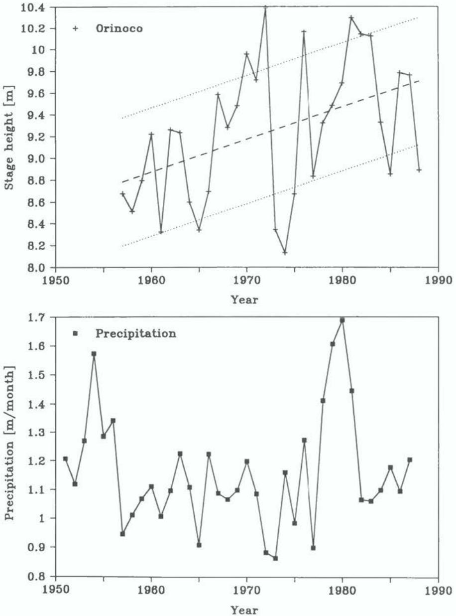
**Fig. 8.5** Orinoco. Time-series of annual mean stage height values (m) (1965–1988) at Ciudad Bolivar on the Orinoco and annual mean precipitation estimates (m/month) (1941–1987) at several stations within the Orinoco’s catchment area. The linear trend ( $\pm$  SE of the slope) shown for the Orinoco stage height was obtained by least-squares regression (see Table 8.1).
