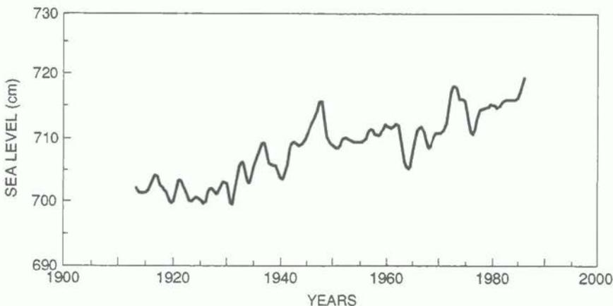
**Fig. 9.7** Time-series of annual mean sea level at Key West, Florida, from the Revised Local Reference data on file with the Permanent Service for Mean Sea Level.
