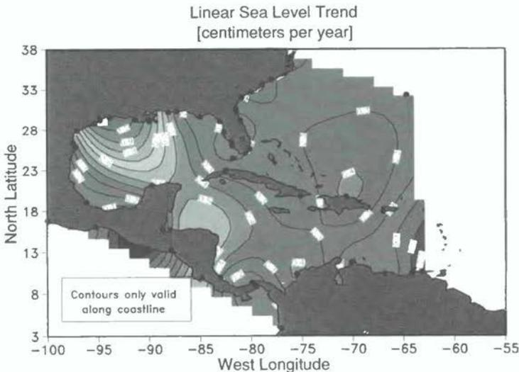
**Fig. 9.8** Distribution of linear trends in annual mean sea level for stations (dots) with more than 10 years of record during the last 60 years. Of the 51 stations used, eight are from the Pacific Ocean and are not included in Table 9.2. See colour plates between pages 210 and 211.
