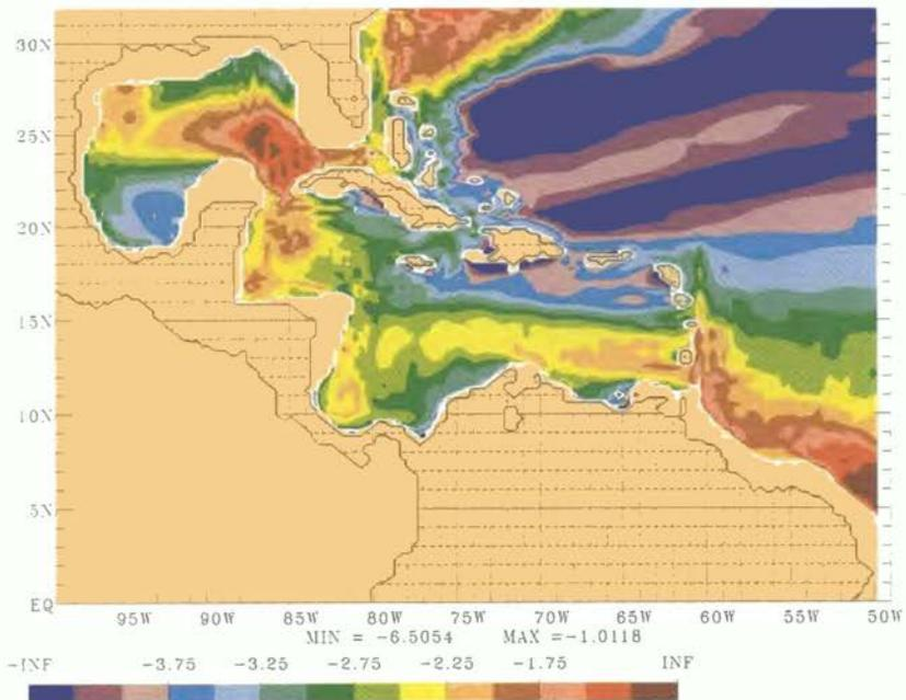
**Fig. 4.1b** Same as Fig. 4.1a except for an open basin with a 15 Sv South Atlantic surface inflow and a high-latitude surface outflow. Maximum kinetic energy is  $0.18 \text{ m}^2\text{s}^{-2}$ .
