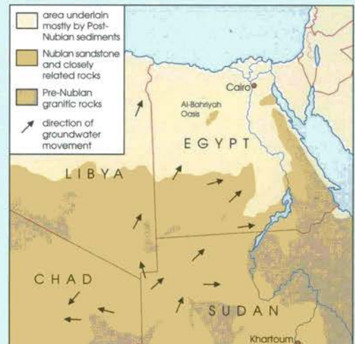
Part of the sub-Saharan fossil aquifer; arrows show the direction of water movement.
