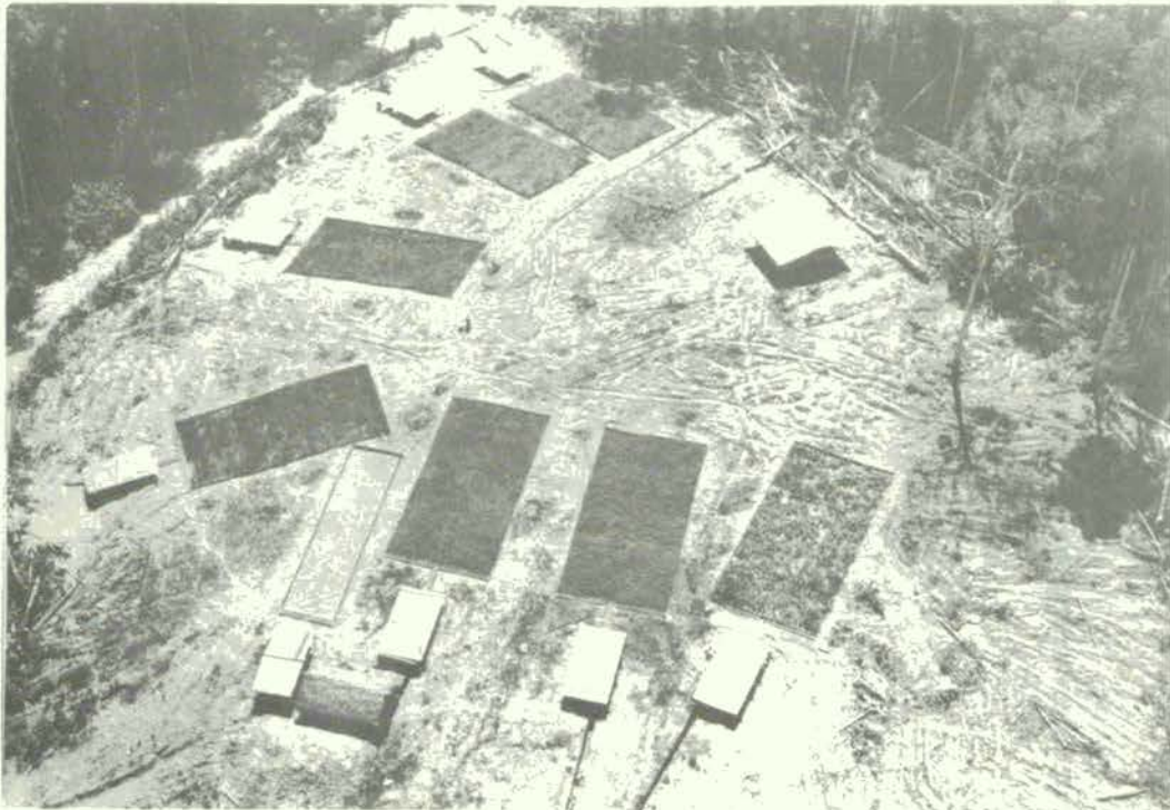
Experimental plots for studying run-off and erosion under different treatments. CTFT-ORSTOM research area, Oyapok drainage basin, French Guyana. Photo: J.M. Sarrailh (CTFT).
