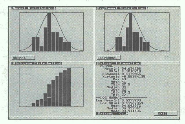
Both normal and lognormal distributions are offered with accumulative information. Standardized boxplot of the distribution showing minimum and maximum, 10th, 25th, 50th, 75th and 90th percentiles can be constructed. These can be used, for example, to compare the longterm distribution with individual year distributions.
