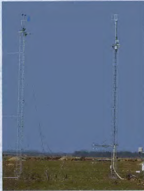
Fig. 4.1 Masts for heat and moisture flux measurements at La Crau.
