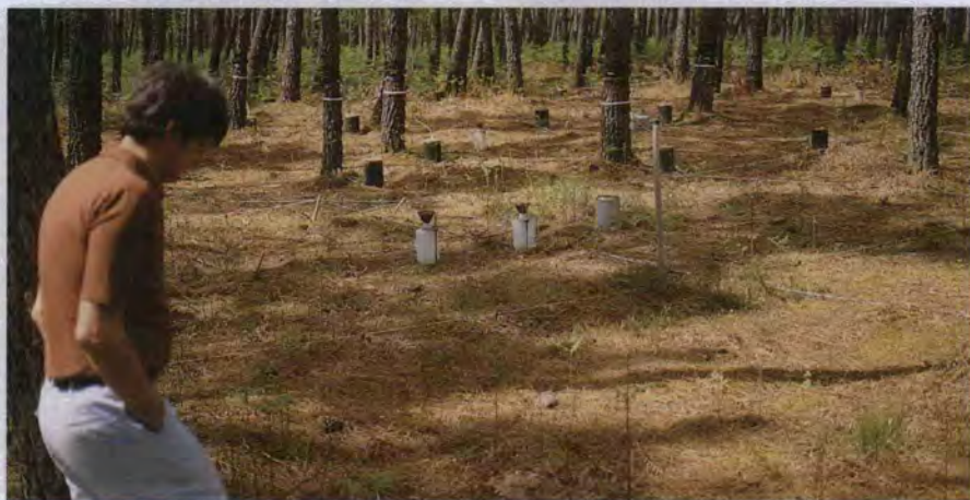
Fig. 4.6 Measurement of stem run-off during HAPEX.
