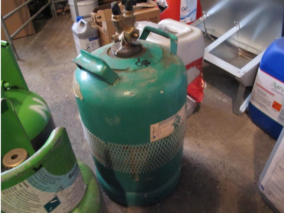
BOTTLE INTERVENED CONTAINING UNIDENTIFIED GAS. LACK OF NUMERATION.
