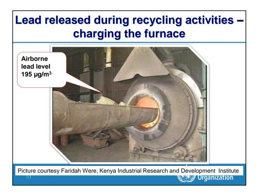
Charging rotary furnace with lead pieces for smelting
