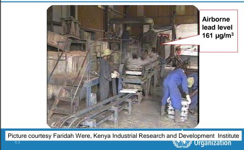
Casting lead into ingots – fumes containing lead can be seen
