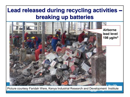
Kenya, formal sector. Breaking up ULABs using axes, the debris is then sorted manually to remove non-lead materials. Release of lead oxide dust and lead particles
