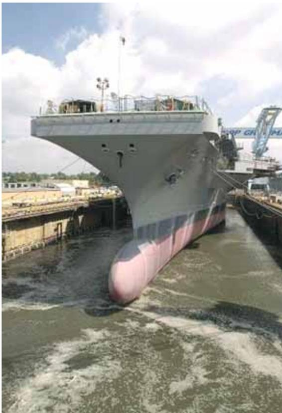
Bulbous bows provide fuel savings from reduced water resistance in naval ships.
