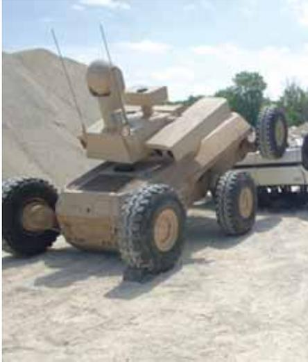
An unmanned ground vehicle. Eliminating the need for a passenger cabin reduces weight, improves fuel efficiency and keeps soldiers out of harms way.
