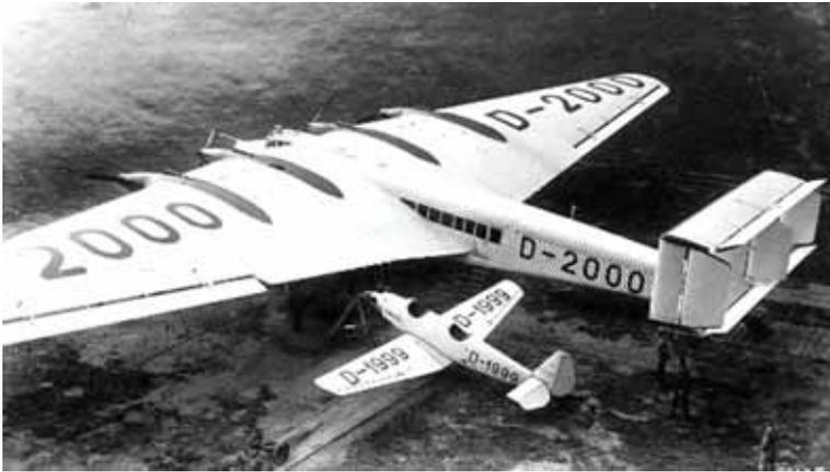
The D-2000, a 1930s precursor to modern blended wing body aircraft, like the proposed design below that can reduce drag considerably thereby improving fuel efficiency.
