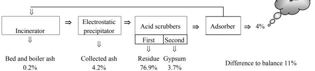
*Figure 5-2* Balance of mercury in a sewage sludge incineration plant of Hamburg, Germany (Saenger et al., 1999b)
