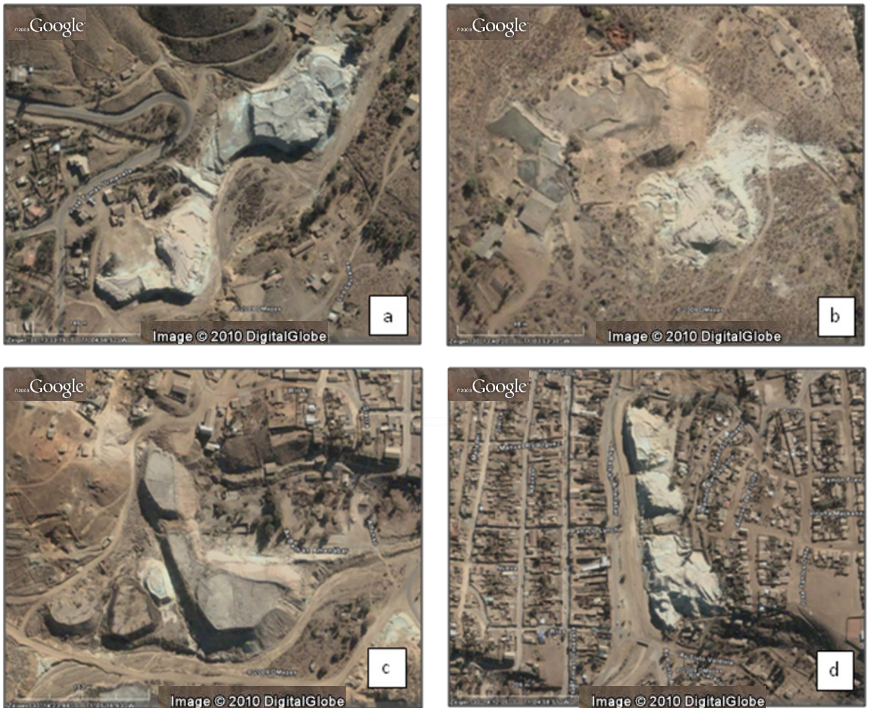
Fig. 11: Erosion of abandoned or poorly maintained flotation ponds and tailings dumps in Andacollo (GOOGLE EARTH 2010).
