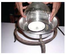
Using retorts, or other mercury vapor capture systems, can reduce mercury losses by as much as 95 percent.
