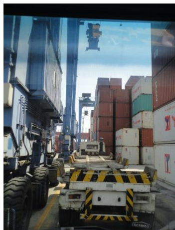
Container from the container yard is lifted to the head truck using RTGC
