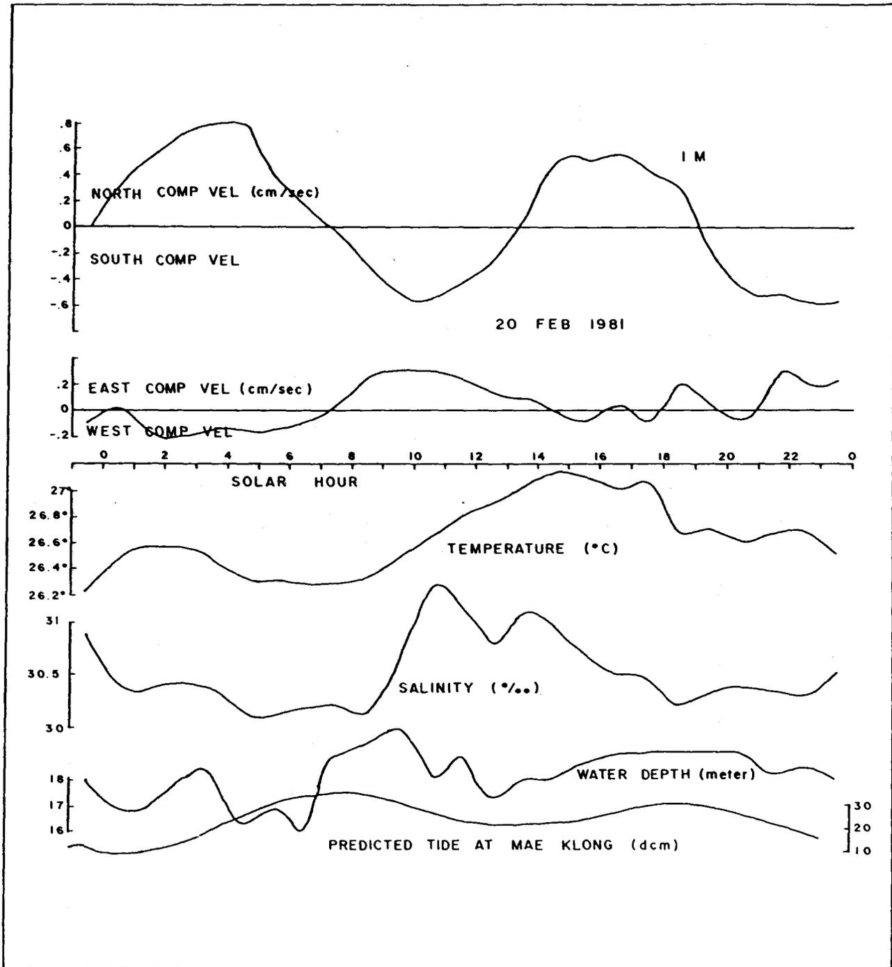
Fig. 1. The variations of some physical properties of sea water offshore of Ban Laem in 25 solar hours at 1 m level (from Siripong and Tamiyavanich 1984).
