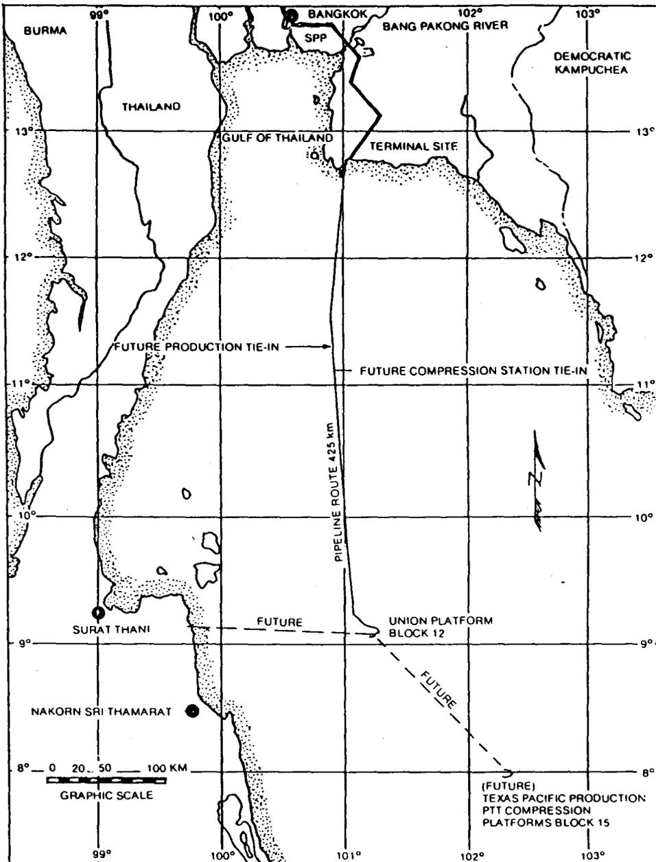
Fig. 6. PTT natural gas transmission system in the Gulf of Thailand.
