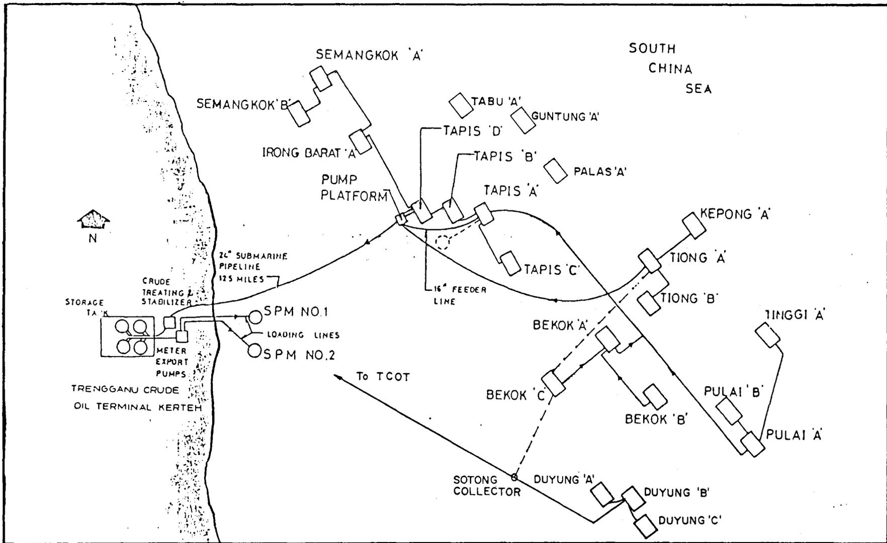
Fig. 4. Schematic layout of production platforms - offshore Trengganu, Malaysia.
