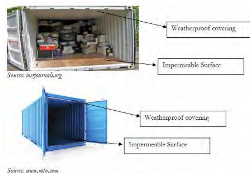
Figure 4.1: Examples of WEEE/e-waste collection system (impermeable surface and Weather proof covering) at a collection facility
