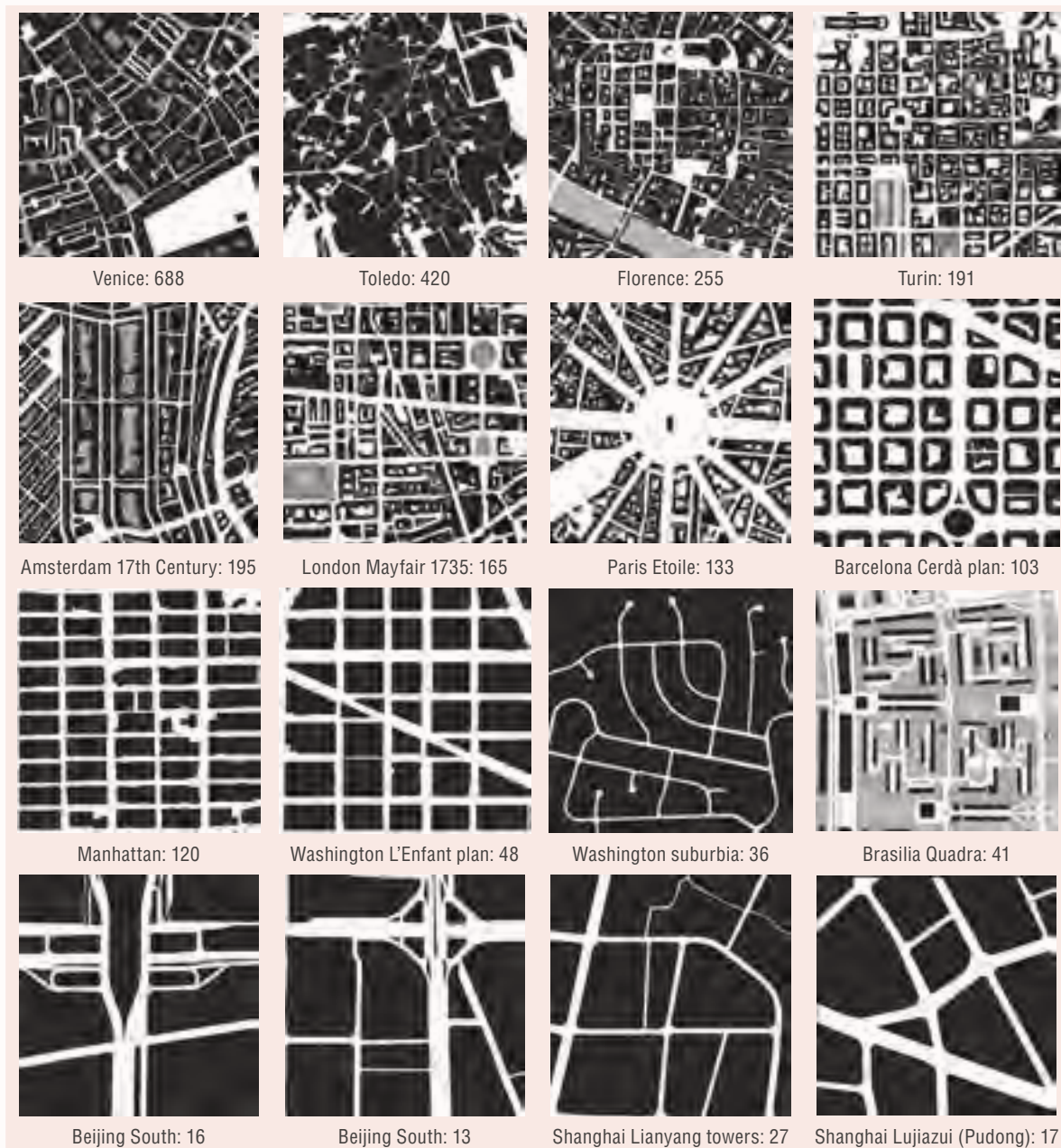
Figure 3.41: Density of street intersections per km 2 in traditional and modernist urban fabrics in 16 cities
