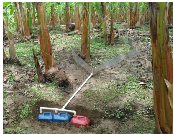
Collection of surface water runoff to be later tested for pesticides residue.
