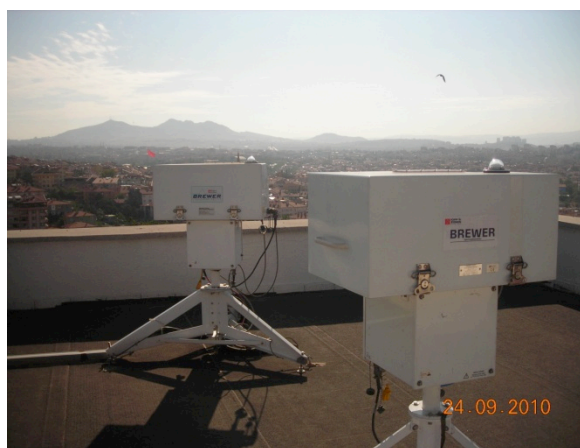
Figure 3. Second calibration of Brewer MKIII #188 with the reference Brewer MKIII #158 in Ankara station.
