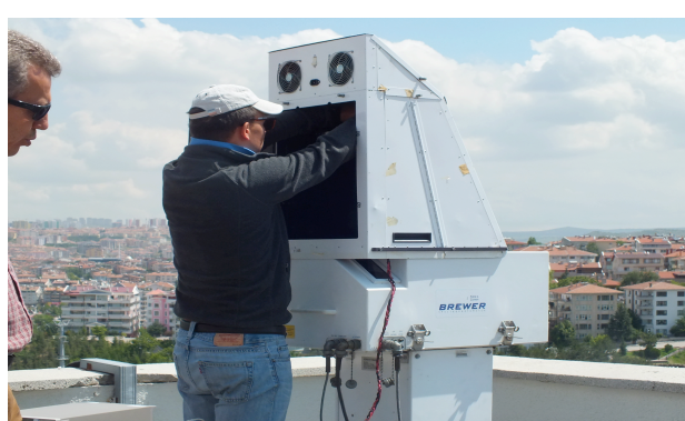
Figure 5. Fourth calibration of Brewer MKIII #188 with the reference Brewer MKIII #158 in Ankara station.
