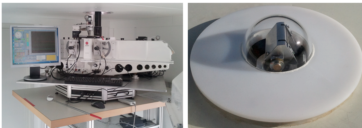
Figure 2: The Dobson instrument is mounted on a rotating table (azimuth) and the entrance prism, protected by a quartz dome, follow the sun elevation (Solar Zenith Angle).
