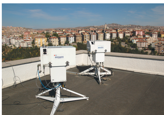
Figure 4. Third calibration of Brewer MKIII #188 with the reference Brewer MKIII #158 in Ankara station.
