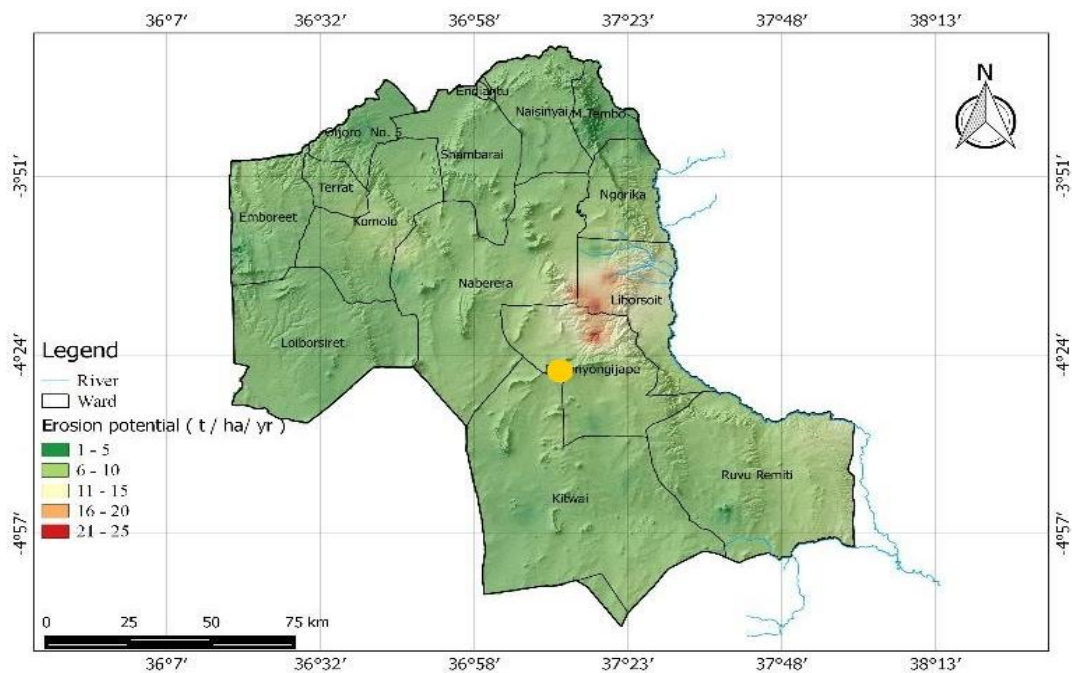
Figure 45: Erosion risk in Simanjiro
