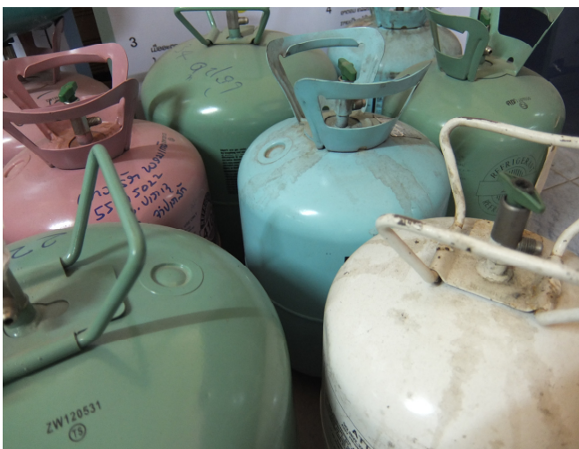
Familiar refrigerant cylinder colours: CFC-12 = white, HCFC-22 = light green, HFC-134a = light sky blue, R-410A = rose
