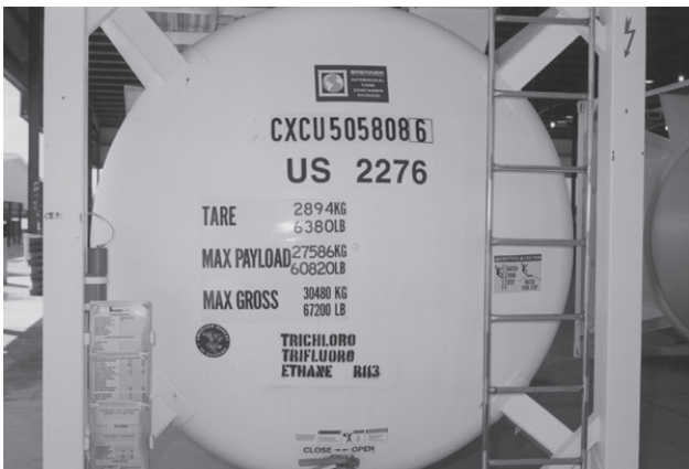
Photo 17 - Front end of an ISO tank (see box for example of ISO tank labelling).
