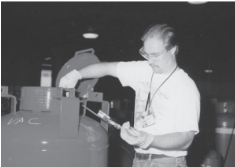
Photo 2. Conducting a temperature-pressure test.
