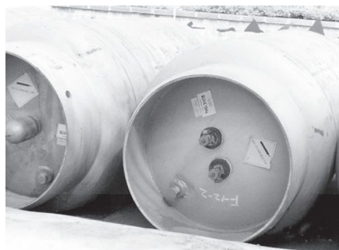
Photo 4. View of the access valves of the small HFC-134a-containing cylinder.
