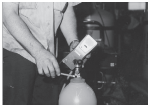
Photo 3. Example of leak detector.
