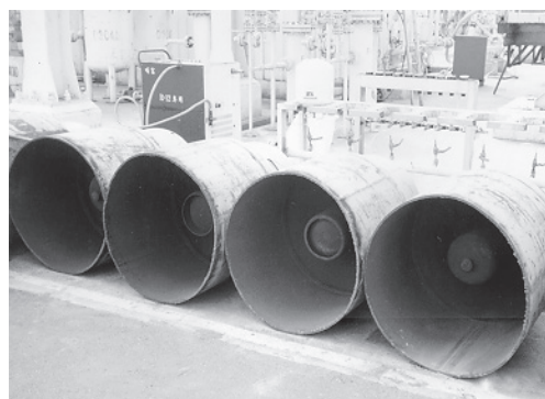
Photo 2. View of the small HFC-134a cylinders after removing the CFC-12 refrigerant and cutting open the main containers.
