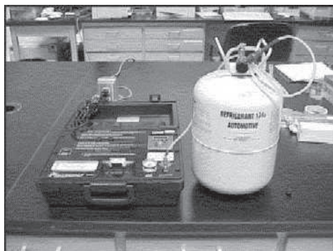
Photo 1. Refrigerant identifier (note that R-134a is not an ODS)
