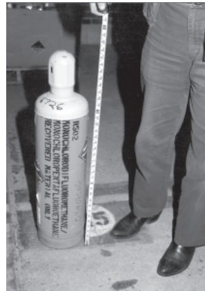
Photo 10 - "Recovered" R-502 (mixture of 49 per cent HCFC-22 and 51 per cent CFC-115) cylinder.
