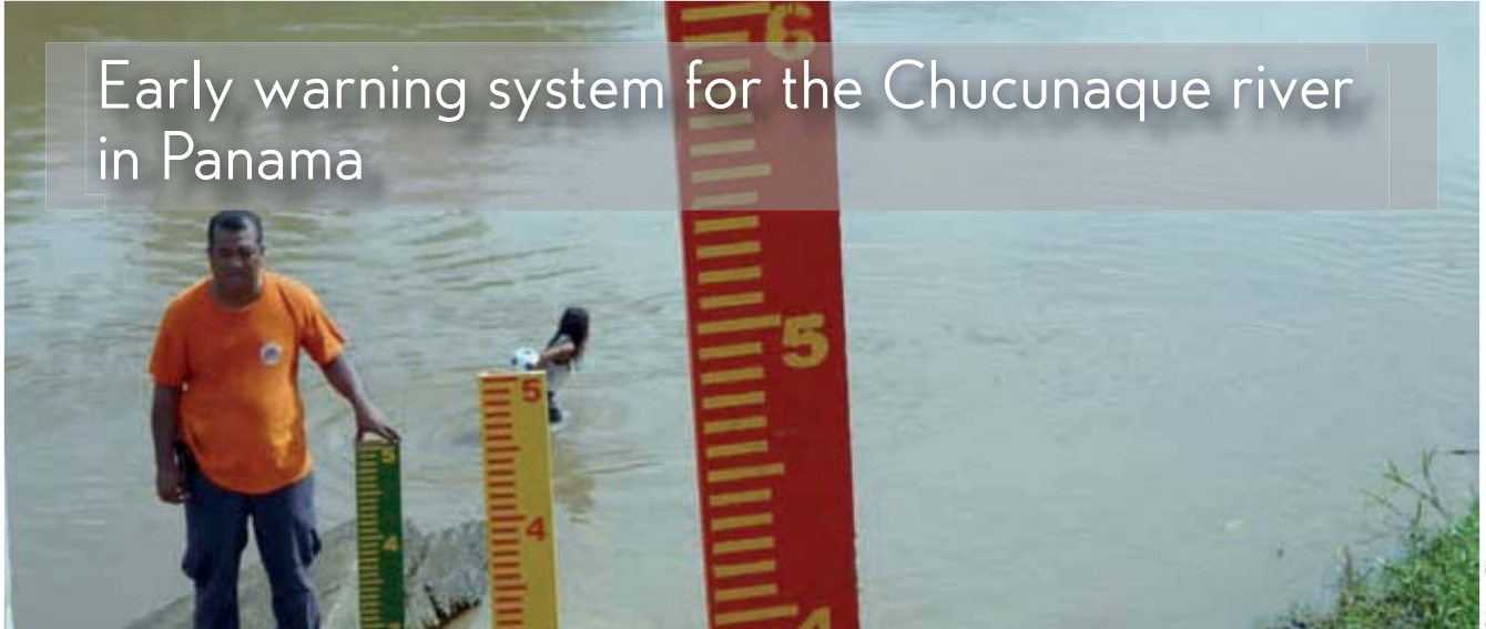
Installation of a limnometric scale in the Chucunaque River around the El Salto community, Panama
