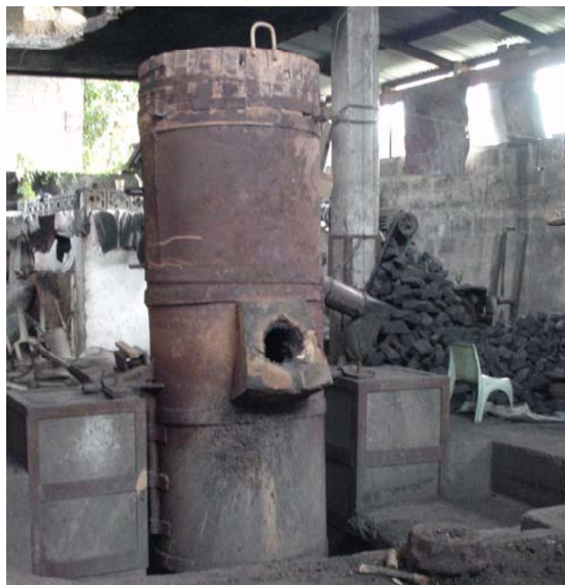
Figure 3: Locally Fabricated Drum-type Furnace
