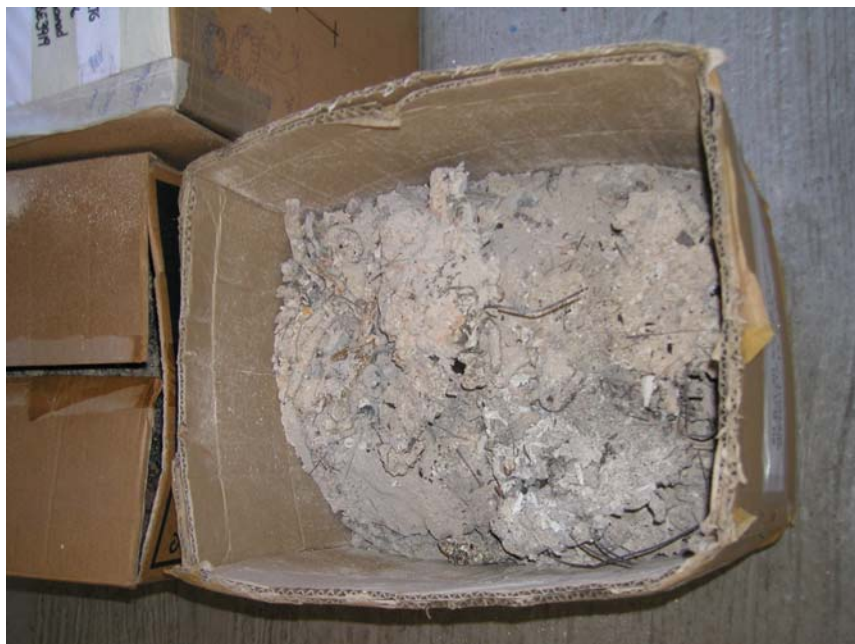
Picture 3: The bottom ash of MWI at RIPAS ready for disposal
