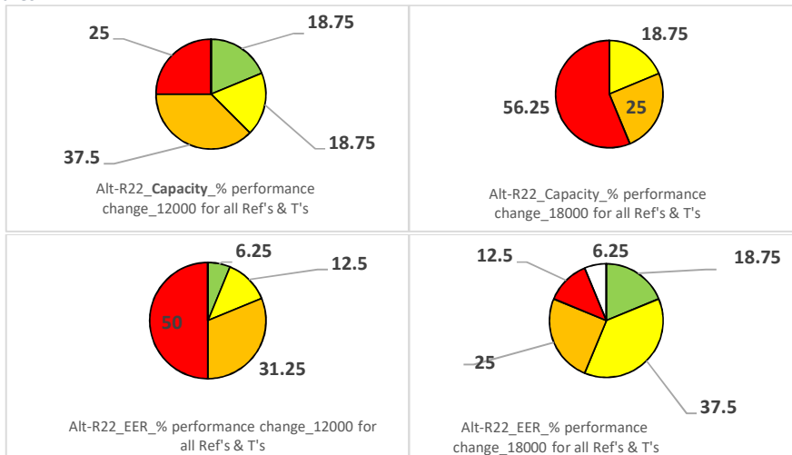
Figure 8 capacity and EER Performance of HCFC-22 alternatives for each category across all refrigerants and all testing temperatures
