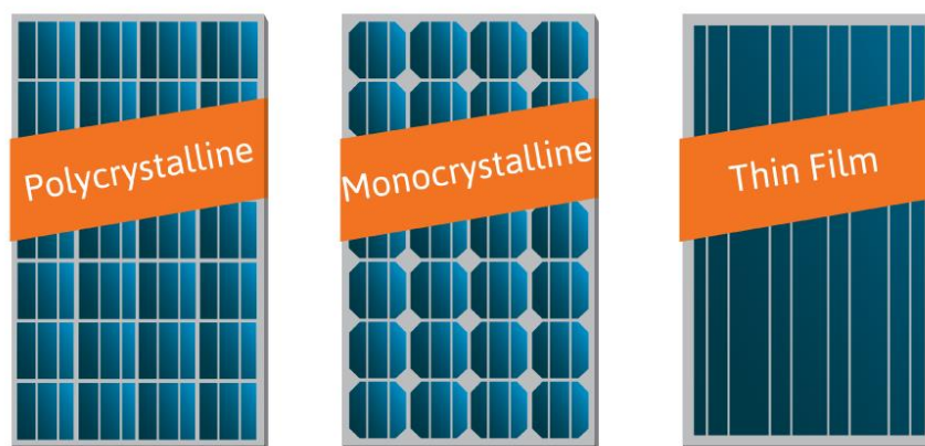
Figure 5: Types of solar PV most common panels (My Solar Quotes , 2016)
