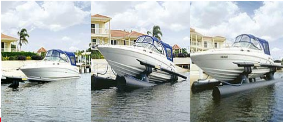
floating hydraulic boat lift
