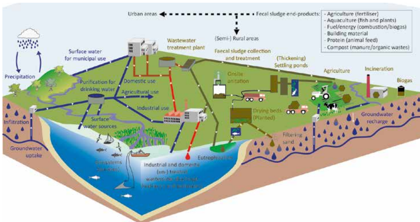
Figure 7. Hydrologic and drinking water cycle, wastewater and faecal sludge collection, treatment and reuse (Source: This report).
