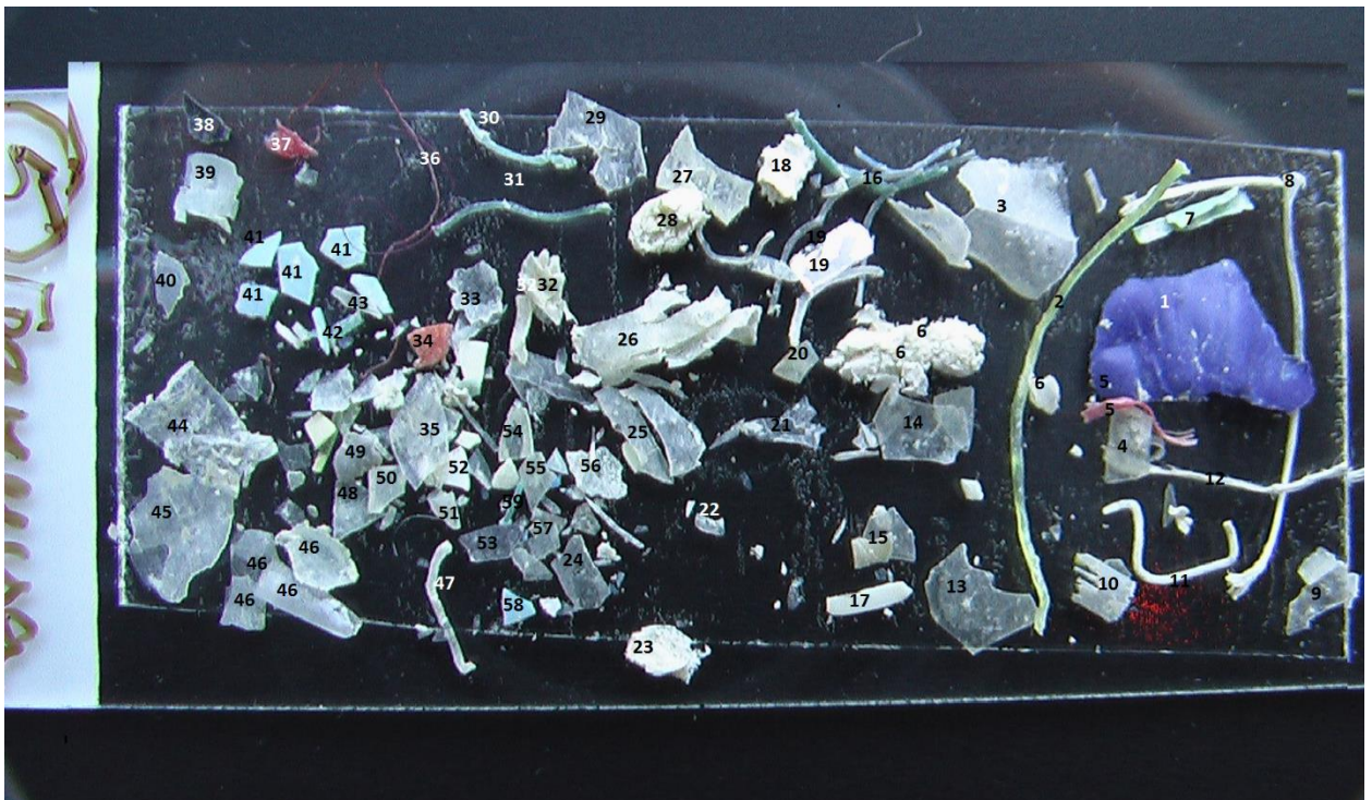
Fig. 2 a) suspected plastic particles in a sample from coastal water near Tumen River estuary prepared for spectra identification (4x magnification)
