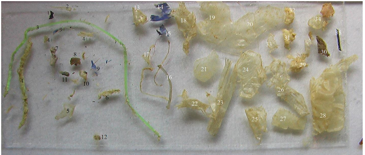
Fig. 2 b) suspected plastic particles in a sample from Razdolnaya/Suifenhe River prepared for spectra identification (4x magnification)
