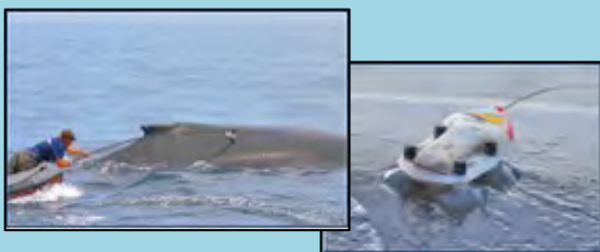
Placing a digital recording tag on a humpback whale. The D-tag records depth and body orientation (pitch, roll, heading).
