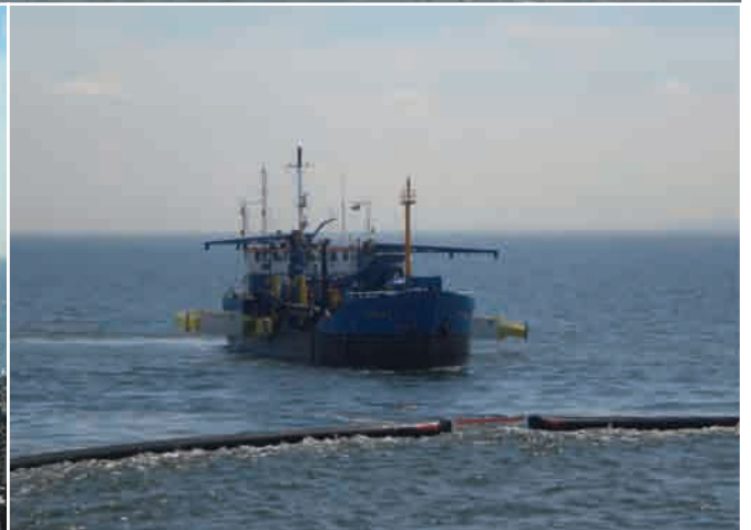
Top: GDC Vlaanderen and Frans Naerbout manoeuvring to form an Open U configuration. Inerballast III with sweeping arms manoeuvring to the position behind the Open U for the simulated collection of oil.
