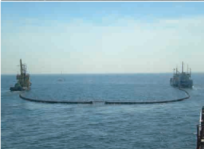
Top: GDC Vlaanderen and Frans Naerbout manoeuvring to form an Open U configuration. Inerballast III with sweeping arms manoeuvring to the position behind the Open U for the simulated collection of oil.
