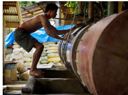
A miner adds mercury to a ball mill at an ore processing facility outside Diwalwal. Image by Larry C. Price. Philippines, 2013.
