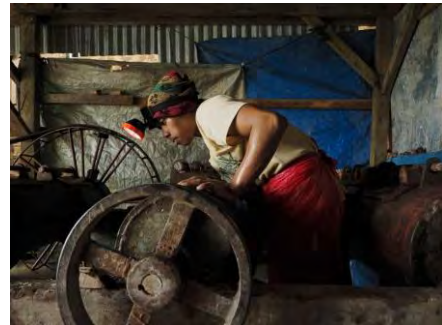
A teenage boy works in a ball mill beneath a house in Diwalwal. Mercury is added directly to the ore in the iron cylinders to make the gold extraction process more efficient. Mercury particulate is released as the ball mills are flushed. Image by Larry C. Price. Philippines, 2013.
