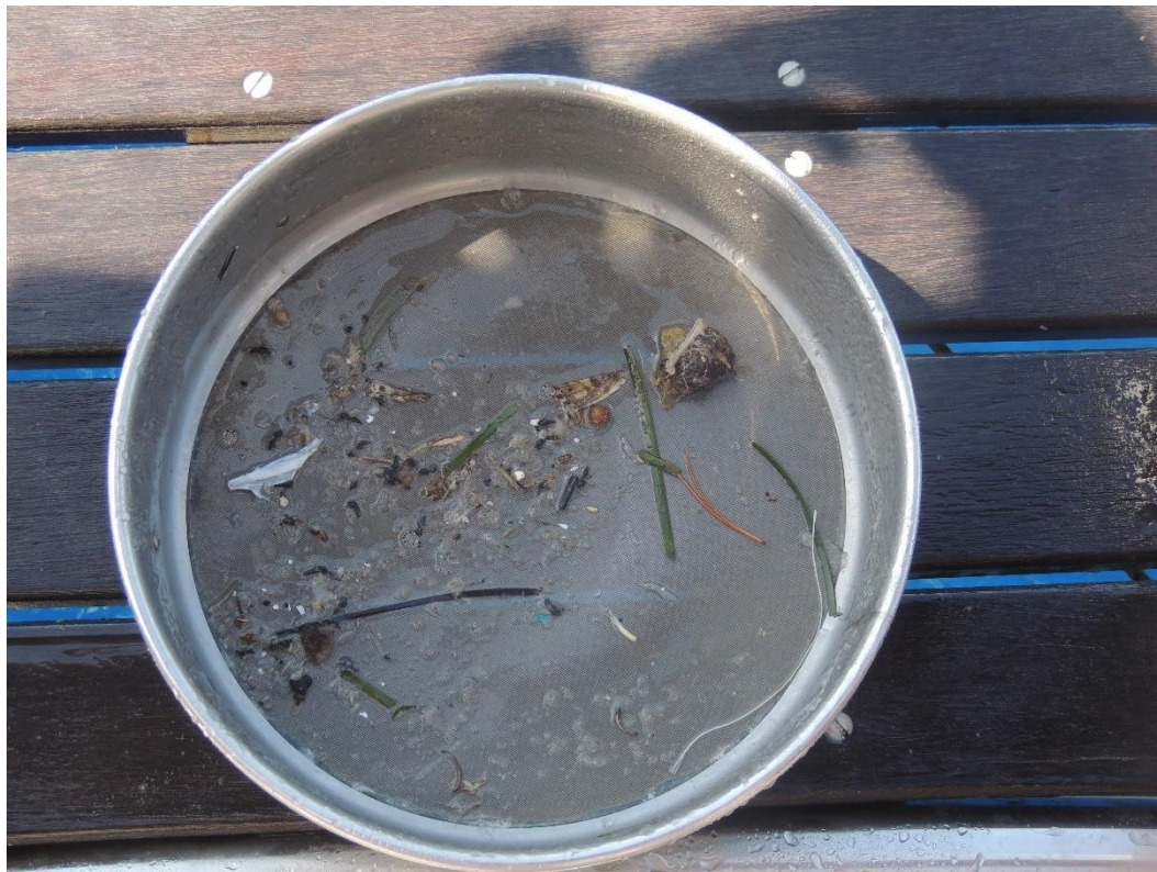
Figure 3: Microplastic and organic matter Collected in a metal sieve just after the sampling (Photo: © Christos Ioakeimidis).
