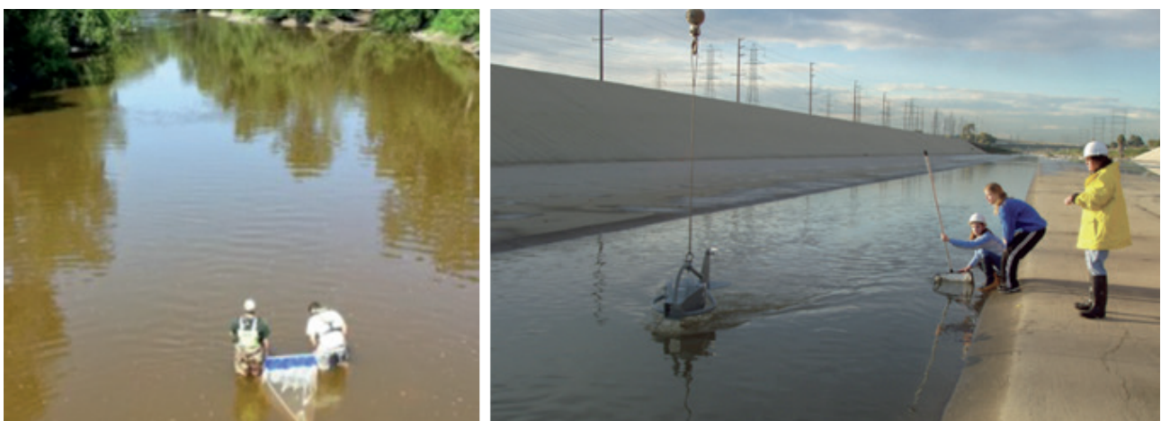
Figure 5.1. Examples of the use of sampling nets in a wadable river (left, Baldwin et al. 2016) and from the bank and a crane (right, Moore, Lattin and Zellers 2011)
