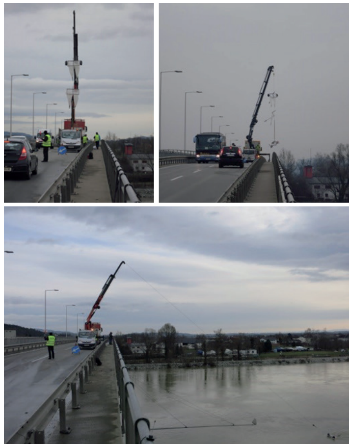
Figure 5.2. Sampling a large river (the Danube) by crane from a bridge. An array of nets is positioned to sample the water surface and the water columns simultaneously (Hohenblum et al. 2015).
