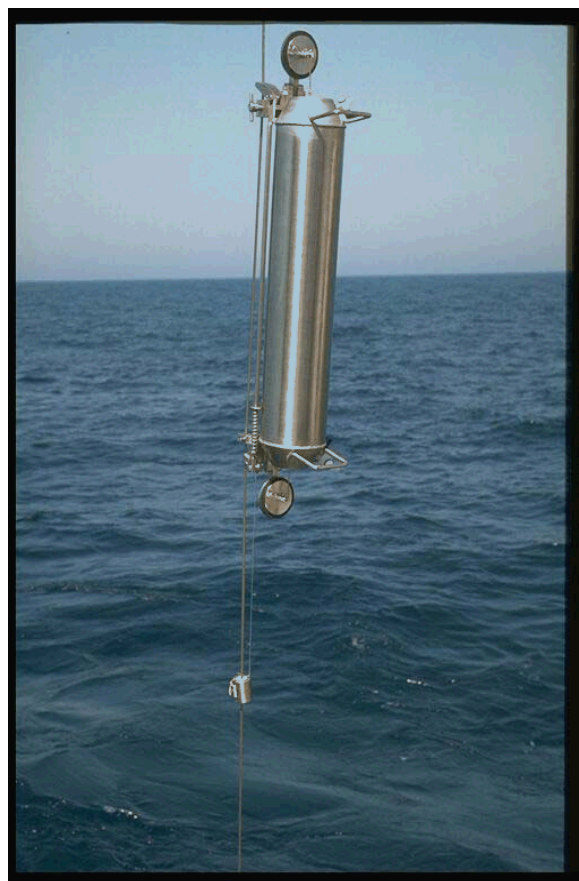
Figure 4 A stainless steel sampling bottle, for subsequent analysis of organic contaminants in seawater.
