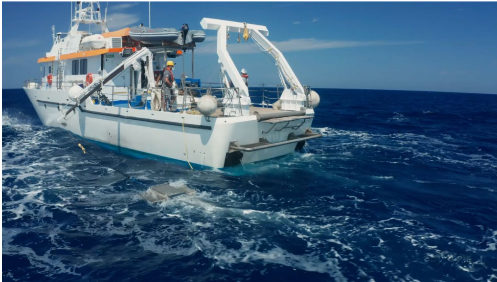
Figure 3: A manta net being pulled from the side of the vessel (Credit © Cecilia Silvestri & Marco Matiddi, Italy)
