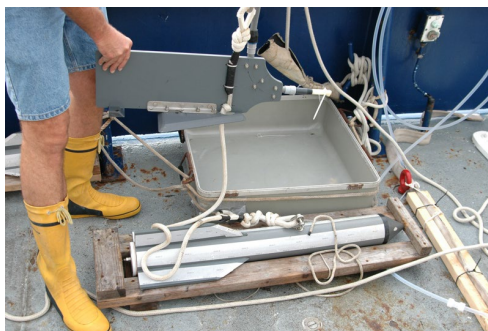
Figure 3. Surface pump sipper/tow fish system (GEOTRACES, 2017)
