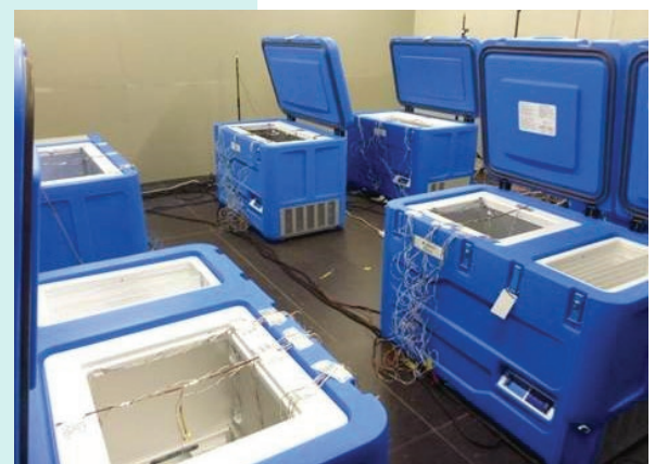
Fig. n°11 : Testing of refrigerators for vaccine storage in the framework of the WHO PQS programme.
