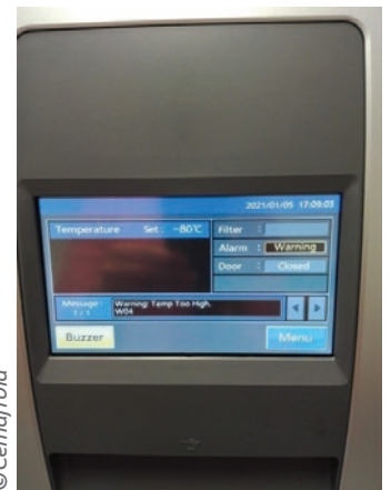
Fig. n°4 : Vaccine storage cabinet at -75^{\circ}\text{C} in the hospital and its control panel
