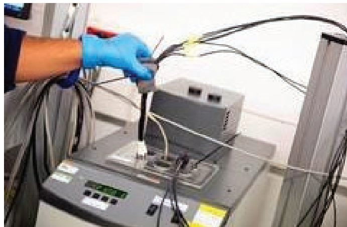
Fig. n°12: Metrological verification of a temperature recorder with external probe
