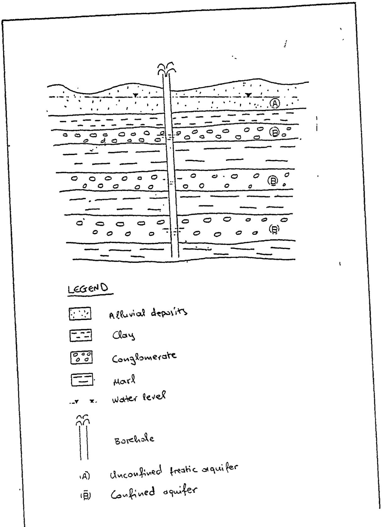
Figure 3 - Hydrogeological conditions of Levantina deposits -
