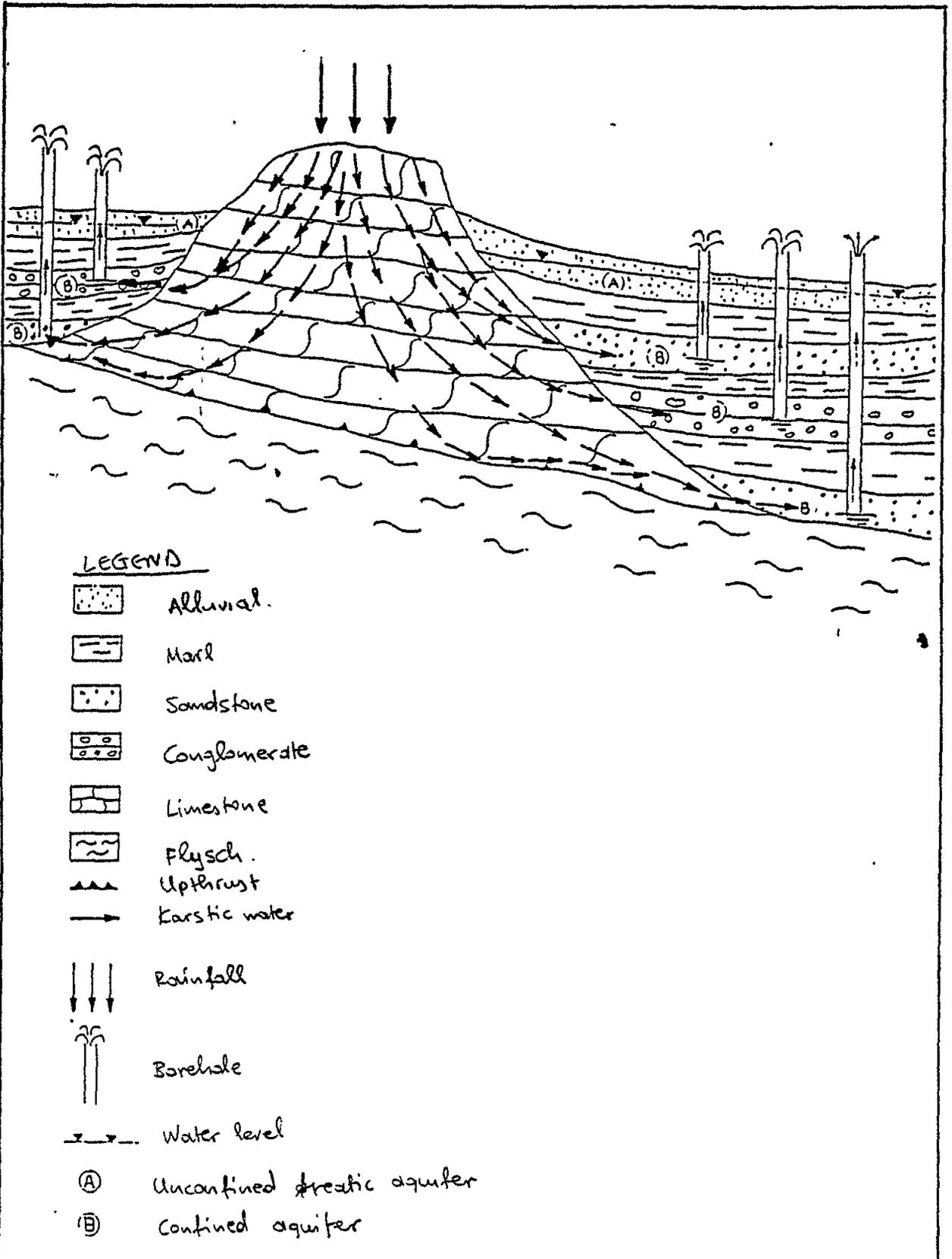
Figure 2 - Hydrogeological conditions of Sgourou formation and undelaying limestone - Archangelos area (Strogillis, 1980)
