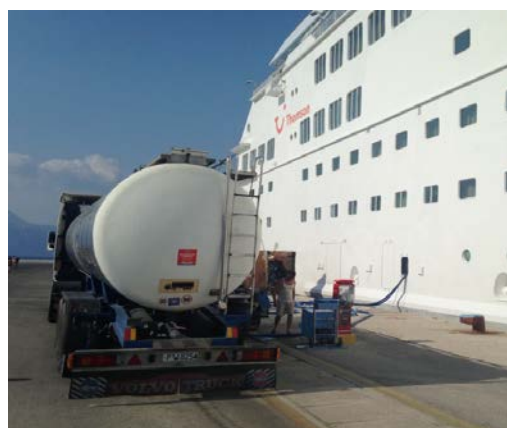
Tank truck collecting liquid waste from a cruise ship (Photo credits: Peter Van den dries)
