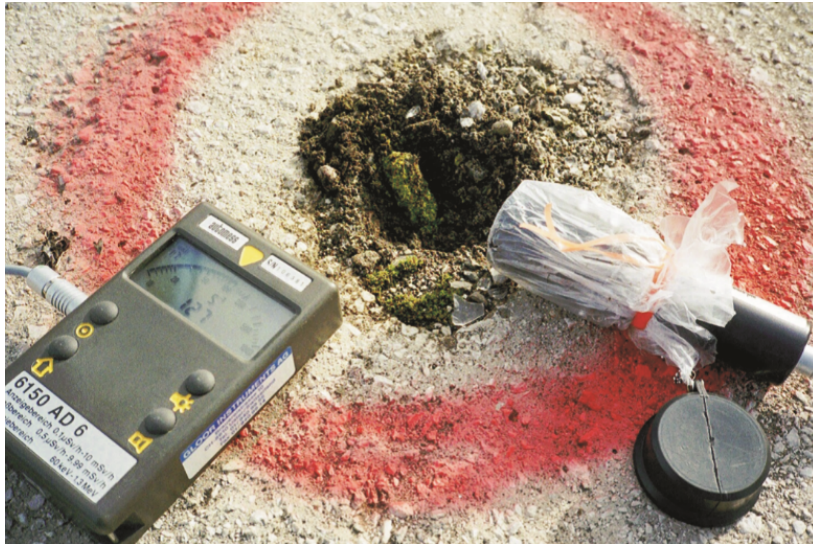
Beta radiation is measured from a penetrator fragment found in the concrete at Hadzici, 2002, UNEP.
