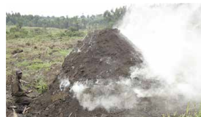
Figure 6: A producer makes charcoal through pyrolysis of the roots from freshly felled trees using a Kasisira (earth-mound kiln technique) in Kyegaliro, Mityana district, Central Uganda (October 2021). Photo credit: Catherine Nabukalu
