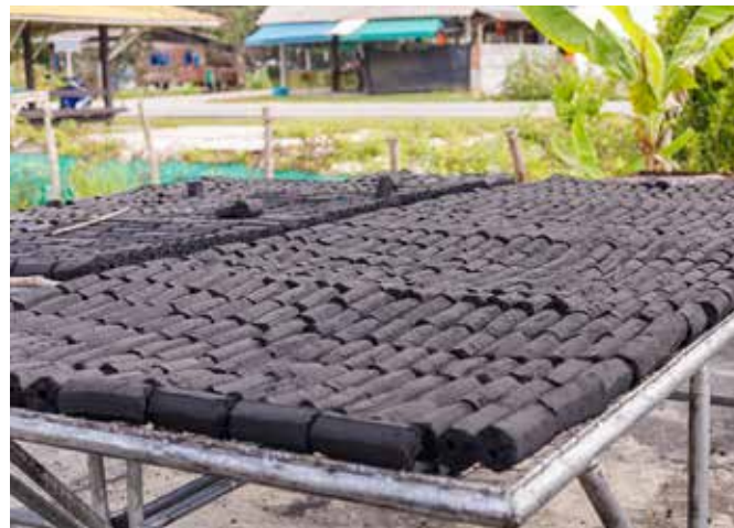
Charcoal briquettes made from coconut shells drying in the sun Photo credit: Shutterstock/phongwit phojurai
