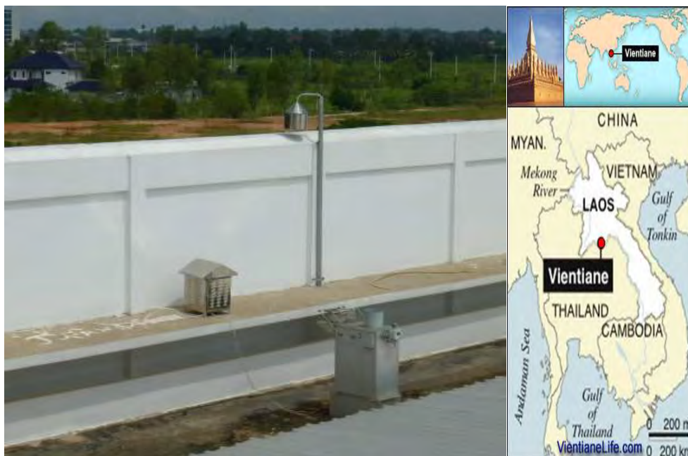
Figure 1.1. Monitoring station for wet and dry deposition.
