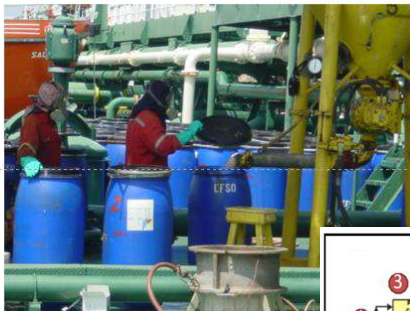
APVAC – NASH VACUUM PUMP/VACUUM HOPPER SLUDGE LIFTING TECHNIQUE
