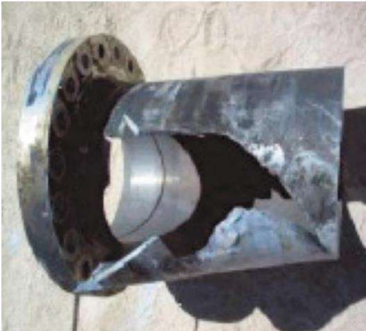
Figure 12 Metallurgical failure caused by liquid mercury
