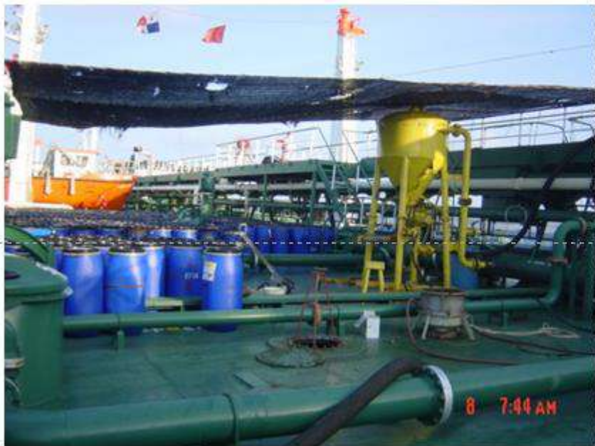
APVAC – NASH VACUUM PUMP/VACUUM HOPPER SLUDGE LIFTING TECHNIQUE
