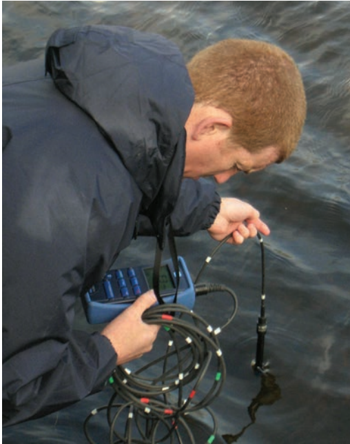
Figure 4.5 Measuring electrical conductivity in situ using a sensor and recording the values manually from a digital meter. © Deborah Chapman
