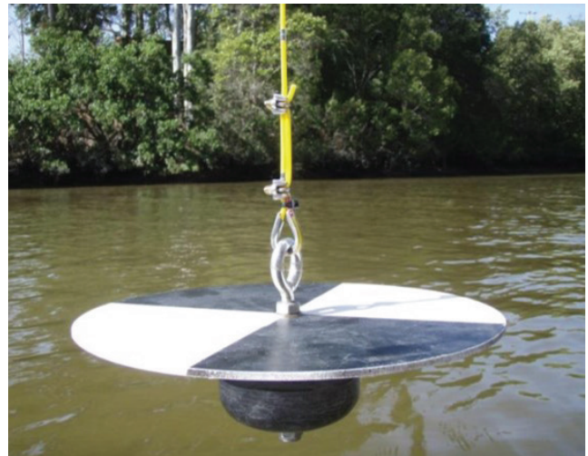
Figure 3.1 A Secchi disc for measuring the transparency of the water (Department of Environment and Science [DES] 2018) By State of Queensland, Licenced under CC BY 3.0 AU
