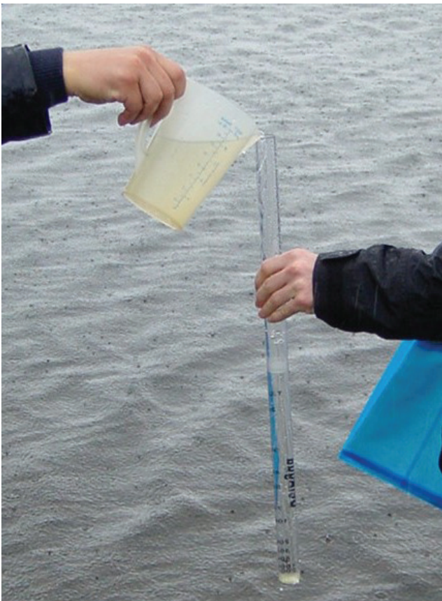
Figure 3.2 A simple graduated turbidity tube is filled with water directly from the water body until the coloured base is no longer visible from above. © Deborah Chapman
