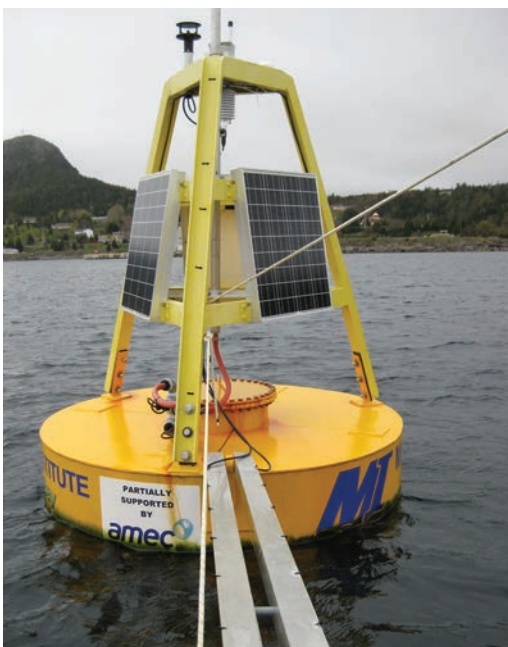
Figure 4.6 An anchored buoy with continuous monitoring sensors suspended at depth underneath. Solar panels provide power for the sensors and telemetry system. © Timothy Sullivan
