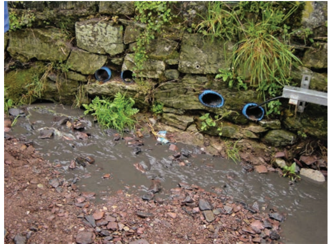
Figure 2.2 Potential sources of influence on the water quality at potential sample sites, such as this highly turbid drainage, can be determined during a preliminary field survey. © Deborah Chapman
