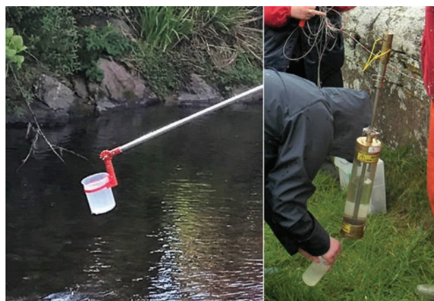
Figure 4.1 Left – a simple dip sampler on an extendable pole. Right – emptying a sample taken from a discrete depth with a Ruttner sampler. © Deborah Chapman
