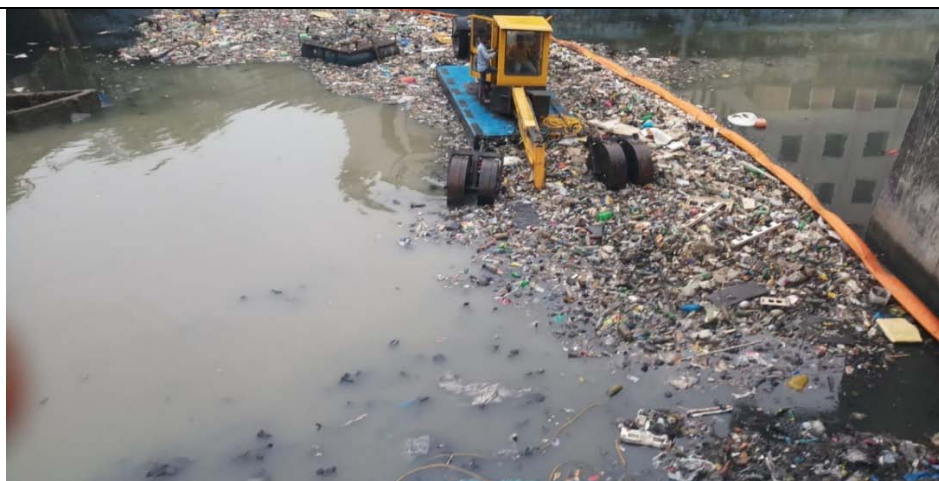
Trash Boom Machine for collection of Floating trash in rivers and mangroves
