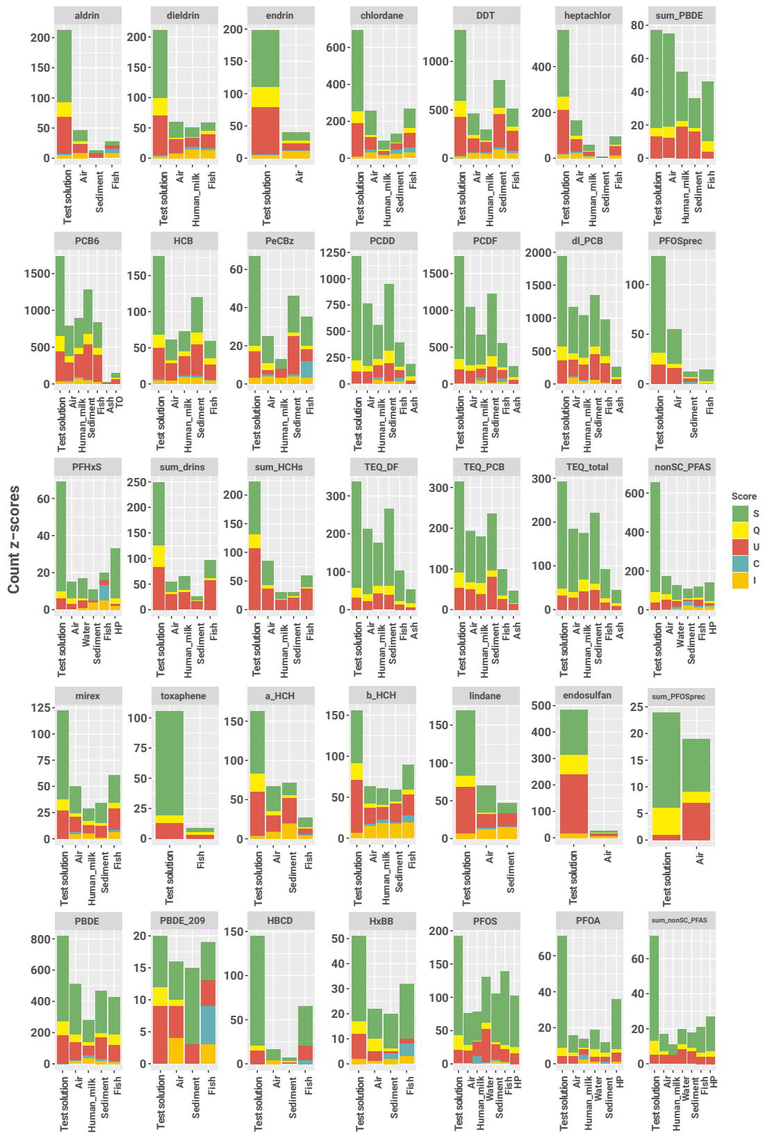
Figure 21: Performance of laboratories by POP and test matrix, stacked bars (IL1-IL4) (as z-score interpretation with S=satisfactory, Q=Questionable, U=Unsatisfactory, C=Consistent, I=Inconsistent)
