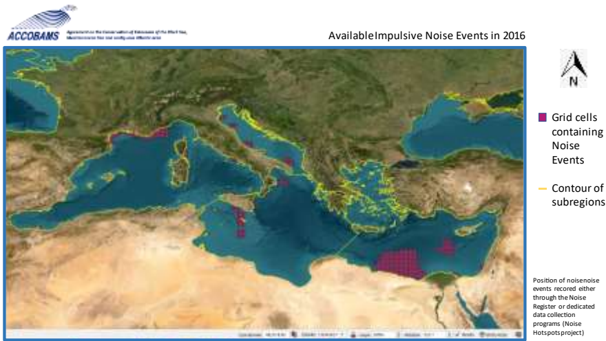
Figure 4.8.1. Impulsive noise events data for 2016. Each purple cell indicates the position of impulsive noise events, meaning that the impulsive noise emissions occurred during at least 1 day in that cell
