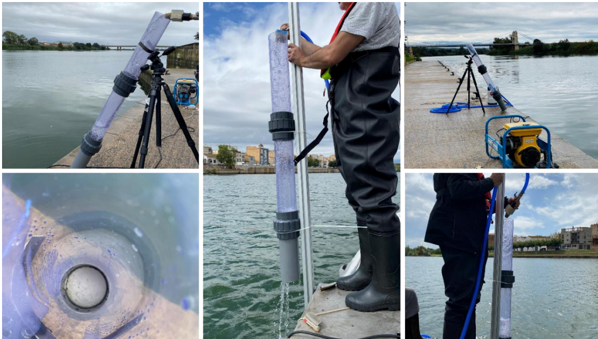
Figure 15: Custom-made set up for the deployment of the series of different filters during the sampling operations (© CEDEX,2021).
