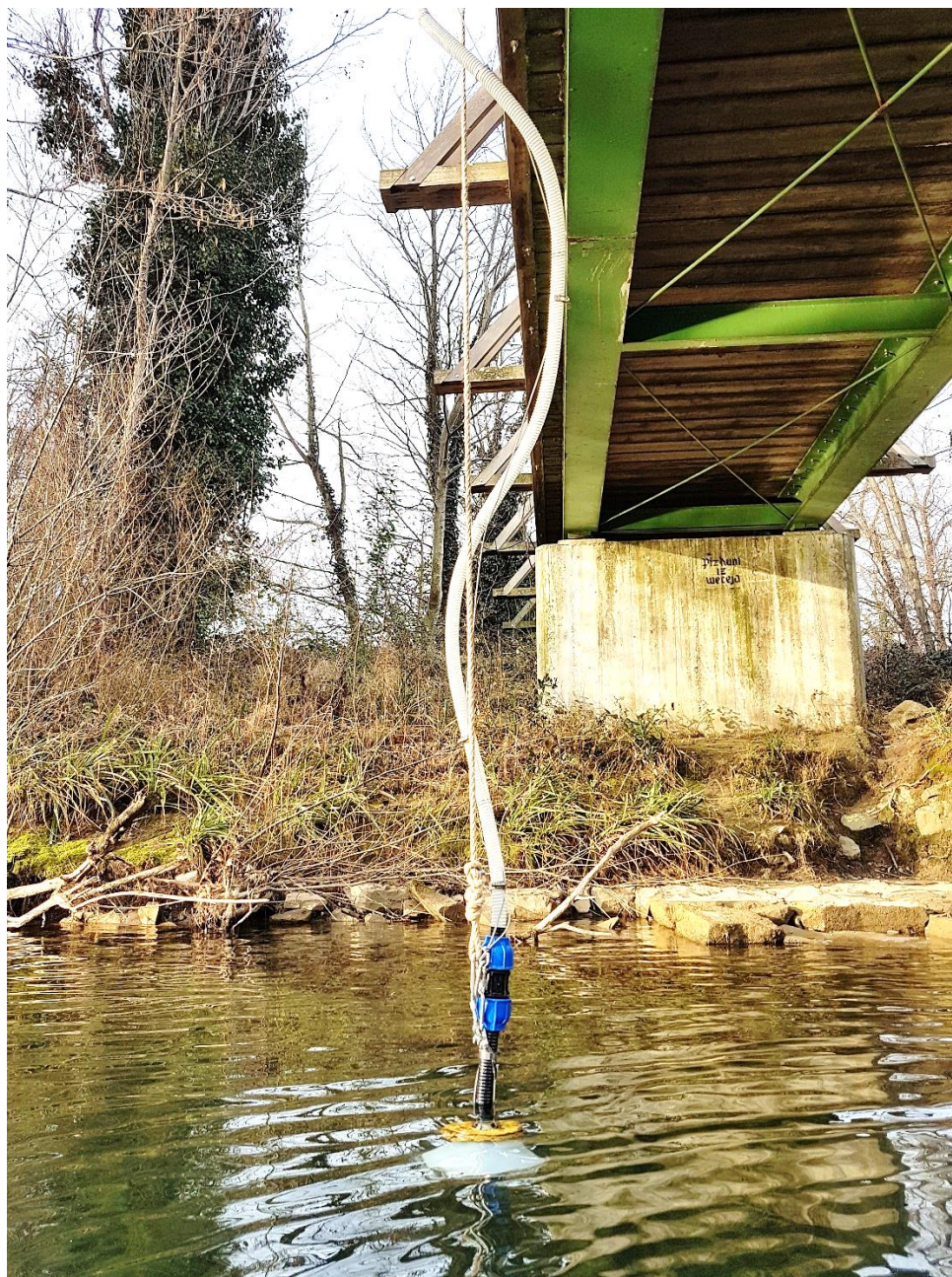
Figure 17: Sampling microplastics from a bridge, using a water pump (© IWRS, 2020).
