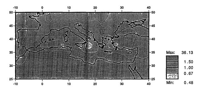
Fig. 2.9 Annual control run precipitation (above, mm/month) and modelled-to-observed precipitation ratios (below): GFDL GCM
