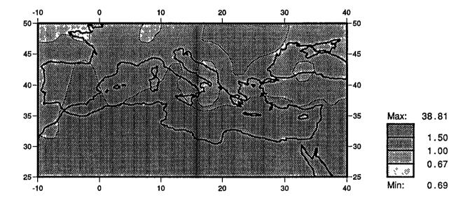
Fig. 2.12 cont. Autumn control run precipitation (above, mm/month) and modelled-to-observed precipitation ratios (below): UKMO GCM
