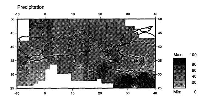
Fig. 4.4 Variance explained (%) by the regression equations estimating summer station temperatures and precipitation in the period 1951-80. Predictor variables temperature and precipitation
