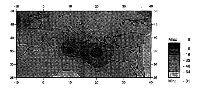
Fig. 2.3 cont. Autumn MSLP control run (above) and control/observed differences (below) in mb: GFDL GCM
