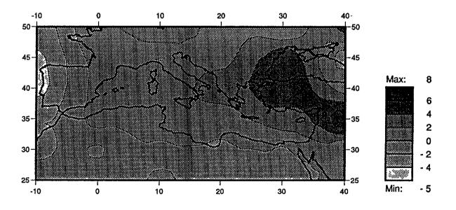
Fig. 2.4 cont. Winter MSLP control run (above) and control/observed differences (below) in mb: GISS GCM
