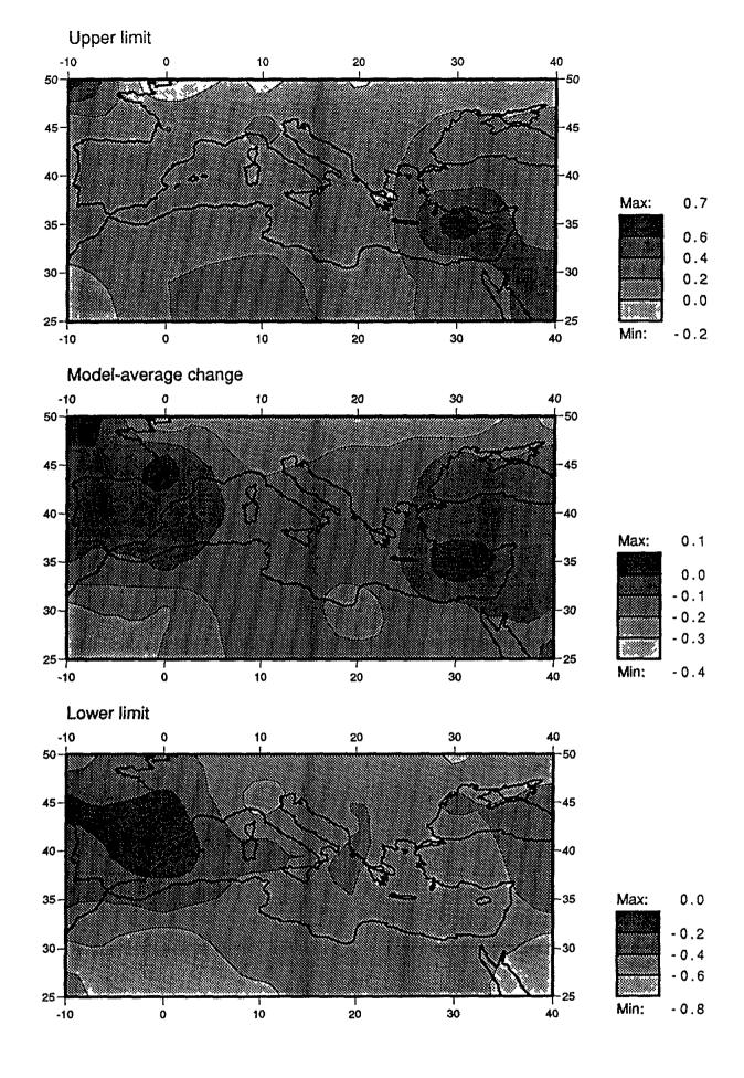
Fig. 3.13 Spring standardized model-average MSL pressure change per <sup>O</sup>C global change, shown with the upper (above) and lower (below) 90% confidence limits (mb)
