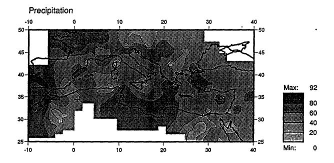
Fig. 4.2 Variance explained (%) by the regression equations estimating winter station temperatures and precipitation in the period 1951-80. Predictor variables temperature and precipitation
