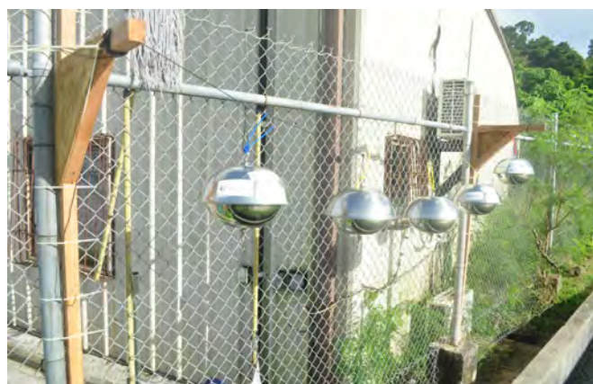
Sampling site for air with PAS/PUF: Palau, © Palau Environmental Quality Protection Board
