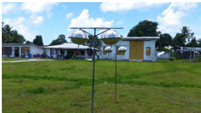
Sampling site for air with PAS/PUF: Tuvalu, Metrological Service Area, © Tuvalu Department of Environment
