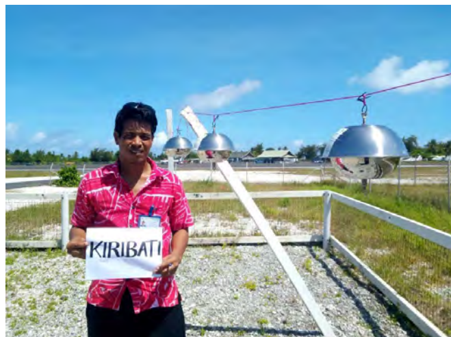
Sampling site for air with PAS/PUF: Kiribati, © Ministry of Environment, Lands and Agriculture
