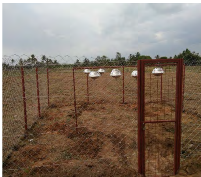
Sampling site for air with PAS/PUF: Tanzania, © Vice President's Office, Division of Environment
