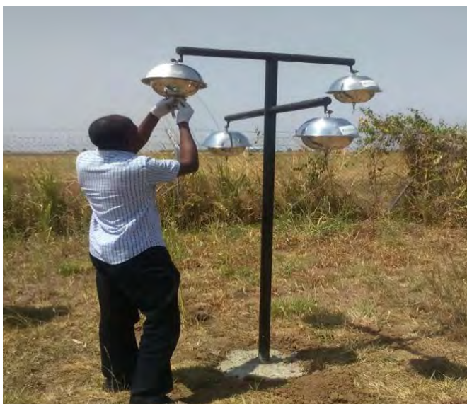
Sampling site for air with PAS/PUF: Uganda, © Directorate of Government Analytical Laboratory (DGAL)
