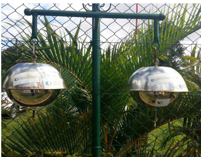
Sampling site for air with PAS/PUF: Mauritius, © Ministry of Environment, Solid Waste Management and Climate Change
